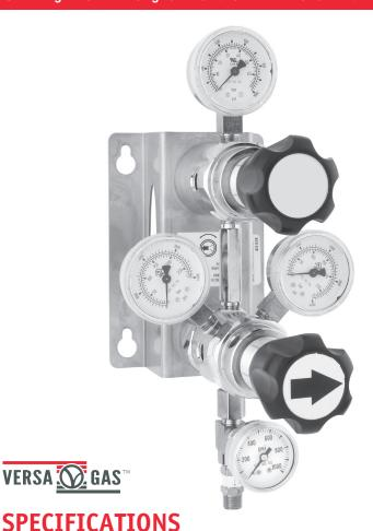
The SG 905 BR / SG 905 SS semi-automatic high purity switchover prevents downtime by automatically switching gas supply from the primary cylinder bank to the reserve cylinder bank. The user resets the primary bank by turning the knob. Manual adjustment of the individual regulators is not required.
